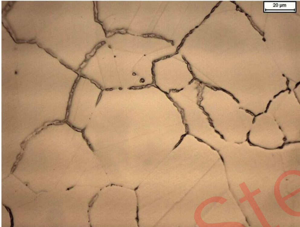
Figure I.6 — Unacceptable microstructure: Coarse and abundant intergranular precipitates. Etchant: 10 g \text{FeCl}_3 , 100 ml ethanol, 30 ml HCl and 70 ml \text{H}_2\text{O}
