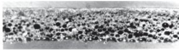
FIGURE 14 CROSS-SECTIONAL FOAMING RATING 4
