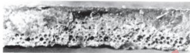
FIGURE 12 CROSS-SECTIONAL FOAMING RATING 2
